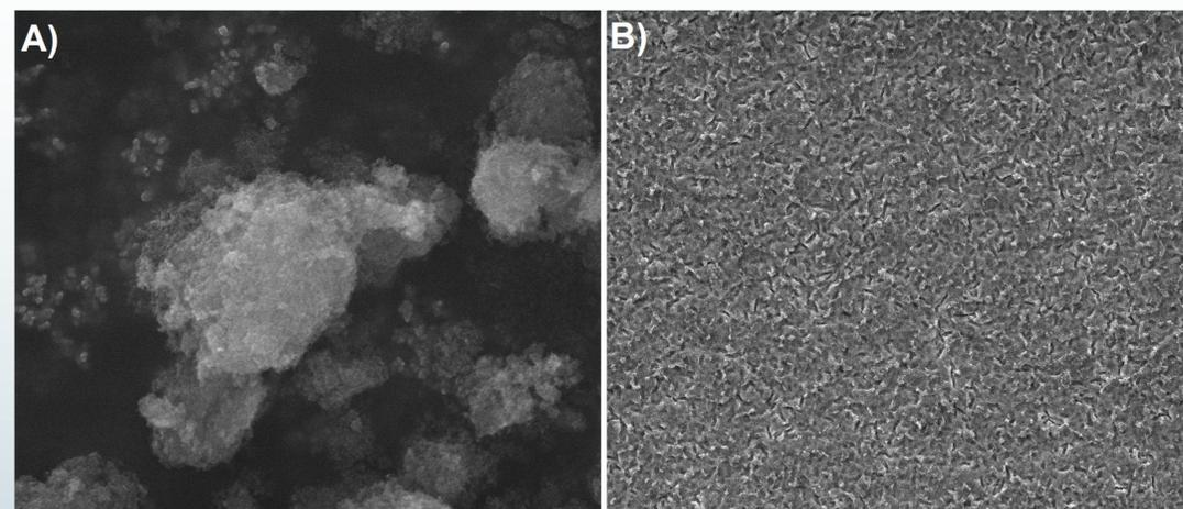
Figure 1: SEM images of AgHAp powders and AgHAp-PDMS/Si thin films.
