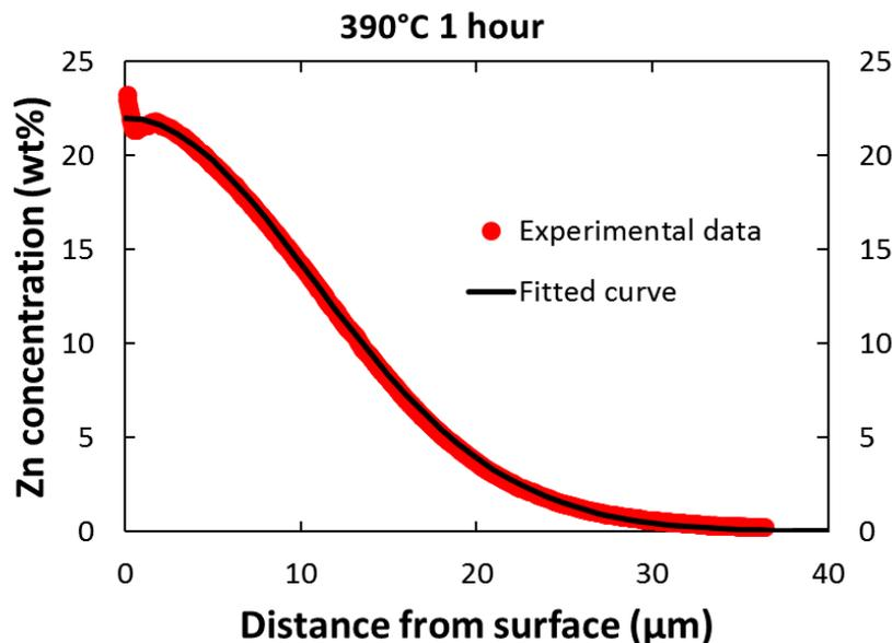
The experimental data (GD-OES profile) was fit by least square fit, by changing the diffusion coefficient  $D$  and maximizing  $R^2$  (coefficient of determination)
